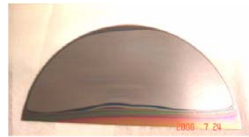
Figure 3. 200mm wafer ashed on the MPP – 5E15, 40KeV As implant on blanket I-line 1.0 micron coated wafer
